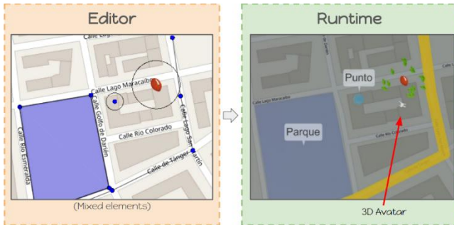
Figure 5: Correspondence of a set of elements in the editor view with the runtime view. Native element on top of the avatar is displaying the discover leaf-based effect.
