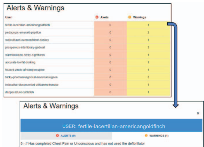
Figure 5. Alerts (messages that appear when a certain condition is satisfied and required immediate action from the teacher) and warnings (also result from a true condition but do not require immediate action) can be configured in the architecture so teachers can receive those notifications in the real-time view. For each user, the number of alerts and warnings satisfied as a result of the user's gameplay appear. User-specific information can be obtained by clicking on a single user, including the alerts or warnings' descriptions that user's gameplay has given rise to.
