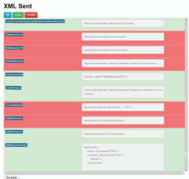
Fig. 4. Teacher visualization of XML sent by the students. This visualization contains 2 columns, one of the username and other with the XML document sent. Teacher can filter valid and invalid documents, and also filter the documents by user name.
