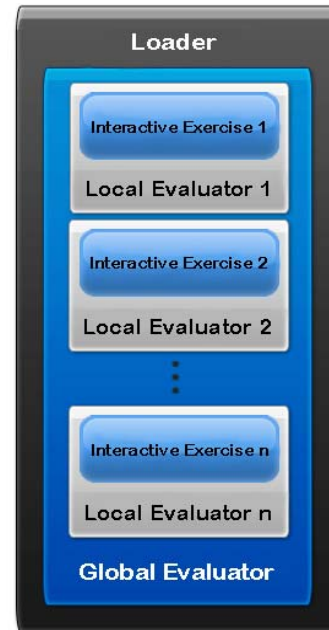
Fig 3. The loader of exercises defines the internal structure of the application executed on the portable game device.
