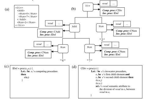
Fig. 7 (a) EXPML document for (6+7)/2, (b) an operationalization of the tree for the document in (a), (c) the IDef *default* invocation procedure, (d) the CDiv computing procedure.
