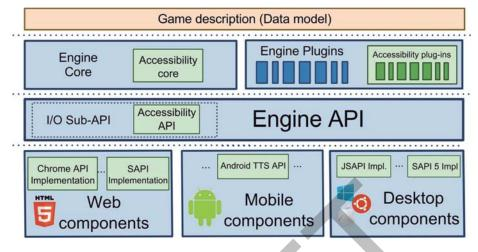
Fig. 1. Architecture of the eAdventure 2.0 engine
